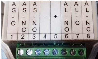
**Plugs AS/C-NC-NO** : Tamper. Connect C-NC for normally close, connect C-NO for normally open.
